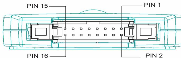
DIN41651-16 pin male connector of the radio modem
