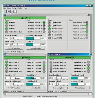
With the functions of the I-LINK PC Pro you can operate systems that are connected to the I-LINK 100 I/O-ports. The visual appearance of the user interface shows all functions at a quick glance. The operating buttons and value fields can be named according to their proper functions. The analogue values can be converted to show the real measured values including the customised low and high levels. These features are helpful if persons other than the operator are monitoring the values and
