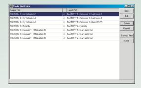
Using the Route List Editor of the I-LINK 100 system software, the Digital and Analogue Inputs can be routed to any Output of the network. In case of a Multialarm, one Input can even be routed to all substation Outputs. For security and to save the workspace, all settings, changes and alarms can be saved to the PC hard disc.
