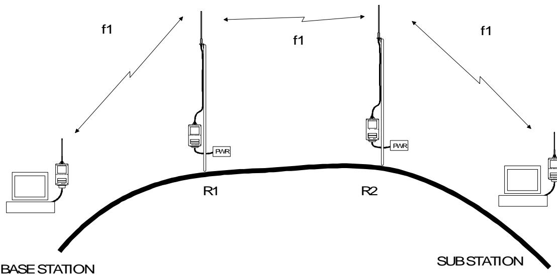
In systems with several adjacent or parallel relay stations addresses should be used. This prohibits moving around of the message and secures that only the determined radio modem receives the message.
