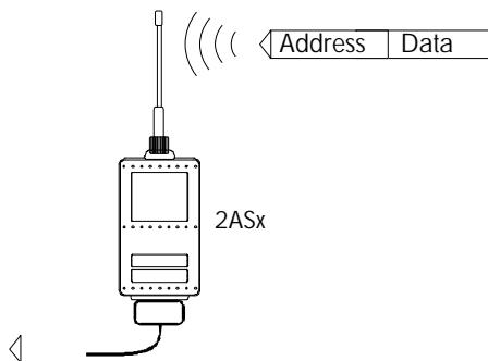
Fig 4 Address of reception has been set ON, but the address of radio modem is different from the address of the received data message. Radio modem will prevent data packet from being transferred to RS-232 interface.
