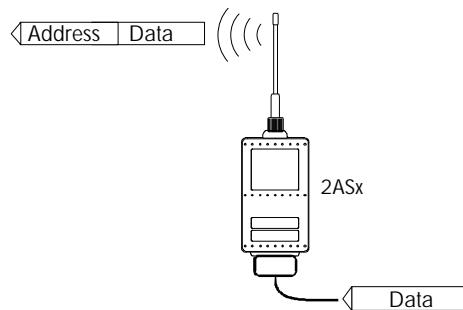
Fig 1 Address of transmission has been set ON.
