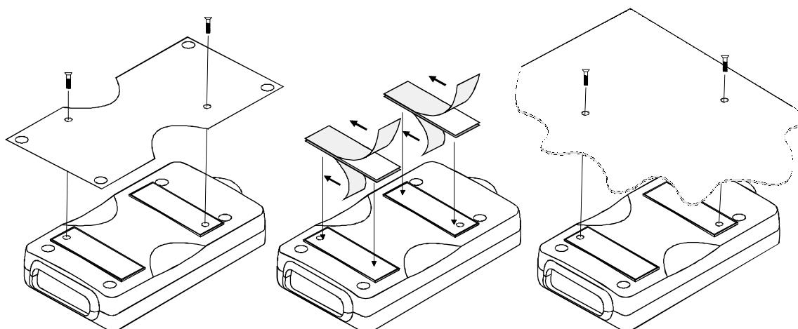
1. By using the installation plate, that should be fastened on the back side of the radio modem. The installation plate can be mounted using the holes provided on installation plate .
