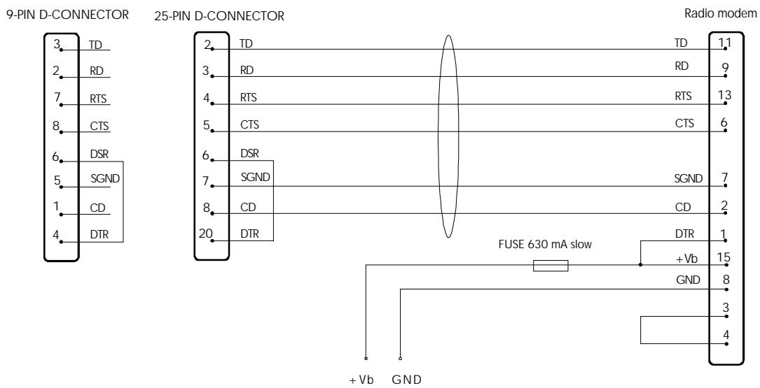
In some systems the radio modem is connected to another data transmission equipment (modem). The lines should in this case be connected accross according to the picture below.
