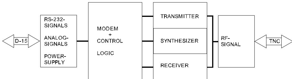
The SATELLINE-2ASx radio data modem consists of a 450 MHz:n transmitter, a receiver, a synthesizer and a modem board, housed in a compact weather resistant aluminium casing. The modem has an RS-232 interface which provides the flexibility to connect it to a wide variety of data networks and terminal equipment.
