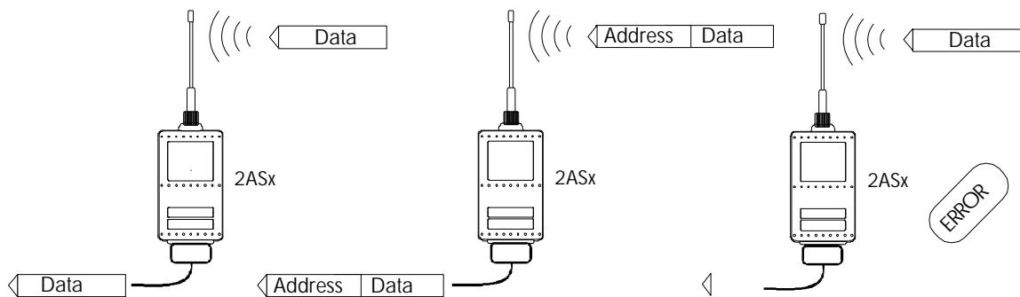
Fig 5 Address of reception has been set OFF.
