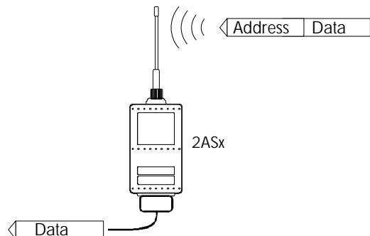
Fig 3 Address of reception has been set ON, and address of radio modem is identical to address of received data message.
