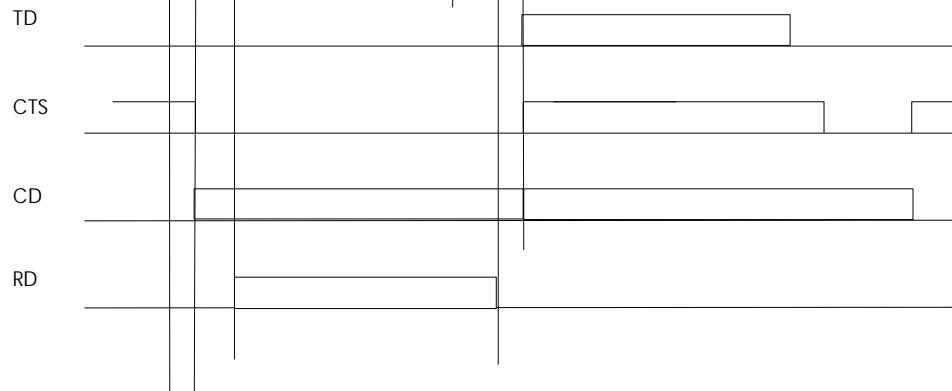
$t_0 = 17 - 20 \text{ ms}$  (typ. 18 ms) delay between TD and RD data
