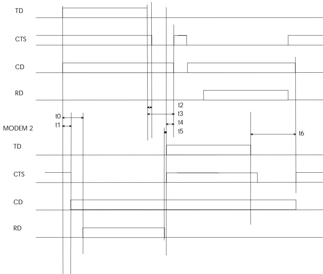
$t_0 = 17 - 20 \text{ ms (typ. } 18 \text{ ms)}$  delay between TD and RD data
