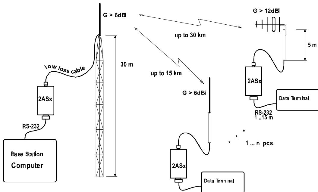
Example of an antenna installation: By use of amplifying antennas and by installing antennas in a high location, long distances can be reached with SATELLINE-2ASx.
