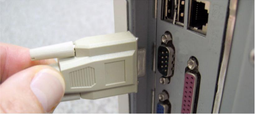
On the other ZN-241G attach the loop-back connector provided as part of the kit.
