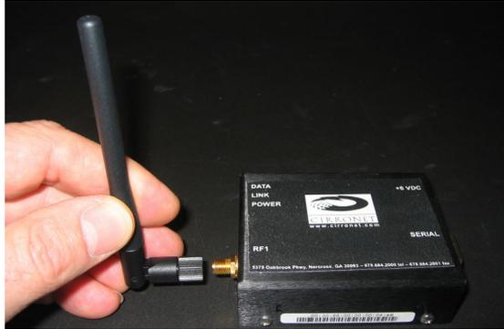
If the folding part of the antenna is not in the right position to stick up above the ZN-241G, hold onto the knurled bottom of the antenna and twist the upper part of the antenna until the foldable part of the antenna sticks up above the ZN-241G. **DO NOT TWIST THE ENTIRE ANTENNA AS THIS MAY DAMAGE THE ANTENNA.**
