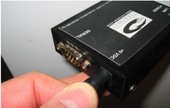
Connect the wall-mount end of the power supply to a wall outlet with either 110VAC or 220VAC. The Power LED on the ZN-241G will come on and after a moment the Data LED will blink. The Data LED blinking means the ZN-241G is looking for another ZN-241G to link to.
