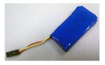
The back-up battery is designed as an optional add-on module and plugs directly on the wire harness. It embeds its own charging circuit, a two cells Lithium Polymer battery and protection circuits in a single housing.
