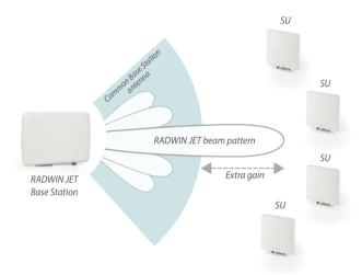
» Improve interference immunity, similar to PtP A result of the narrow beam replacing the wide beam of common sector antennas.
