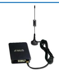
**MLB-G3003 series** is LTE Cat1 modem designed for RS232 and USB communication over TCP/IP via any readily available LTE carrier network. Overall, it offers a more cost effective and time to market solution for bridging remote machine to machine over diverse locations without first having to invest and engineer a huge complex network.
