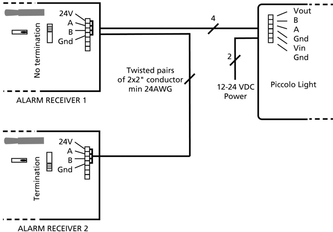
If external alarm receivers are used in an RS485 bus system, be sure to make a termination (resistor termination) of the remotest alarm receiver. To do this, turn the switch on the print: Set the switch to 'Termination'.
