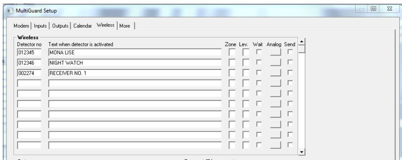
If Piccolo Light is set to monitor the wireless detectors and alarm receiver and has not received signals for 30 minutes, Piccolo Light will issue a 'warning' on the current unit.
