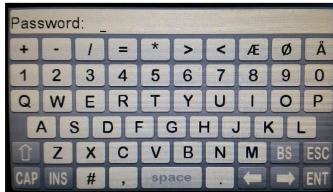
I In 'Password: \_', it is not necessary to enter 1234 the first time you start up, as the unit already knows the default password 1234 in advance. Skip forward by pressing ENT.
