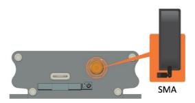
Screw (clockwise) the SMA antenna onto the SMA connector.
