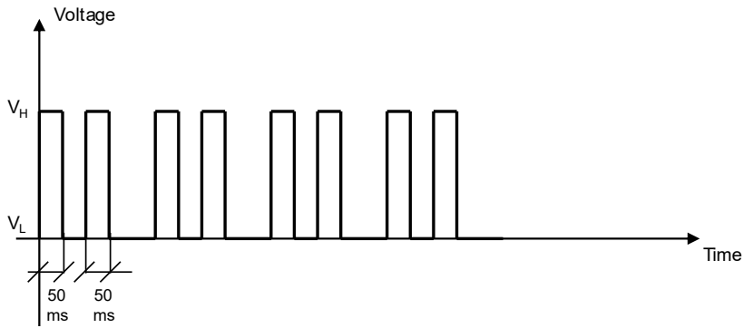
Figure 9: GPIO pin progress for registered roaming 3G
